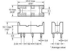
**PCB Mounting Holes** (BOTTOM VIEW)
