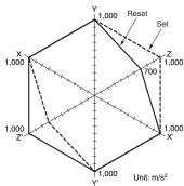
Sample: G6BK-1114P-US Number of Relays: 12 pcs Test Conditions: The value at which malfunction occurred was measured after applying shock to the Shock direction test piece 3 times each in 6 directions along 3
